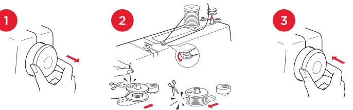
In order to ensure correct bobbin winding, follow the above diagram for correct threading. Use both hands to thread machine around the guide for correct tension. Pro tip: Because different brands of thread unwind in various manners, sometimes it is helpful to lightly hold the thread as it comes off the spool. This will help create smooth and tightly wound bobbins which is important for a good stitch.
