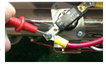
THIS TEST WILL VERIFY THAT ELECTRICAL POWER IS GOING TO THE BOTTOM AND ACROSS THE THER-MOSTAT.
