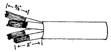
6. Insert all the conductors into the proper wire terminals.
