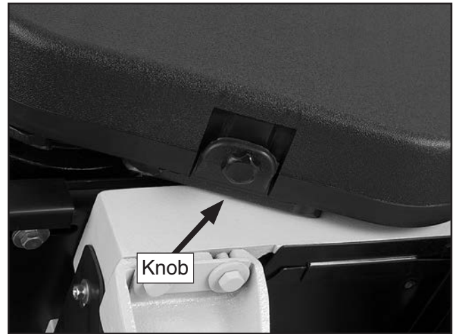
Figure 20. Secured pulley cover lid.
