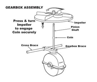
**Step 4:** Install GEARBOX by inserting the PINION SHAFT into hole in center of HOPPER bottom. The word "FRONT" on the GEARBOX must point to Front of the HOPPER.
