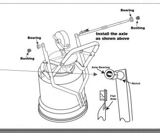
NOW GO BACK AND TIGHTEN ALL NUTS AND BOLTS STARTING WITH FIRST STEP. DO NOT OVER TIGHTEN.
