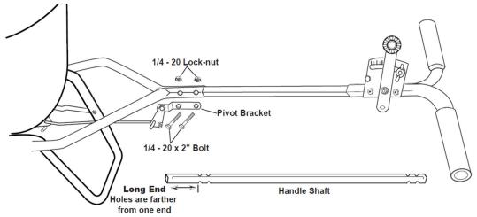
**Step 13:** Install flattened end of CONTROL ROD in to LEVER on GAUGE as shown. Turn to lock in place. Next push LEVER forward to setting "0". Align CONTROL ROD with hole in PIVOT BRACKET, pull LEVER backward to insert CONTROL ROD through hole in PIVOT BRACKET.
