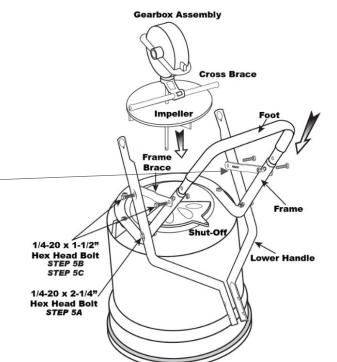
**Step 6:** Slide AXLE into the LOWER HANDLE, then the GEARBOX and into the other LOWER HANDLE as shown above. Next, install AXLE BEARINGS over the AXLE and into both LOWER HANDLES as shown above.
