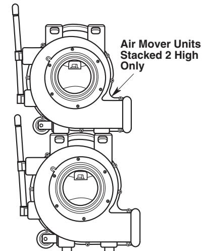
To transport the units in a stacked position, fully extend the bottom Air Mover handle. Grasp handles of each unit firmly, and tilt units backwards and move to desired location.
