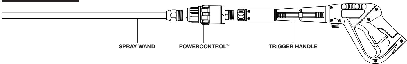
**PowerControl™ connects between trigger handle and spray wand
