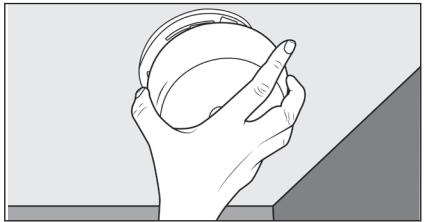
5. Line up the light with the mounting plate and twist the light clockwise until it locks into place.
