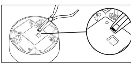
Locate the black rectangular piece in the light. Remove the black rectangular piece with needle nose pliers by lifting up. Once the piece is removed, the light sensor will not work until piece is replaced.
