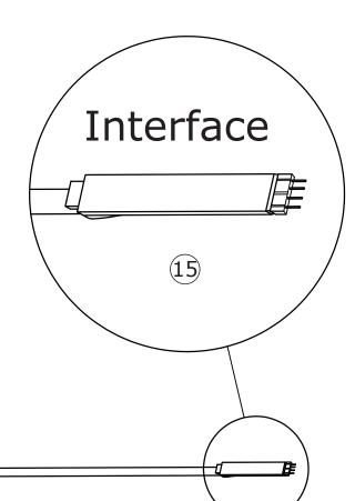
Stick light bar 15 to inside of board 5, 7 and 6 as shown.
