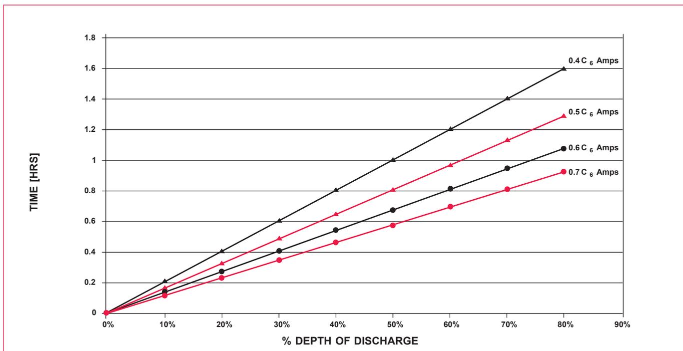
Figure 3 – Recharge time – return 80% of discharged Ah's
