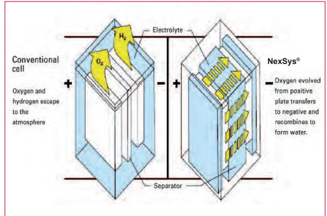
Figure 1 - Principle of the oxygen reduction cycle
