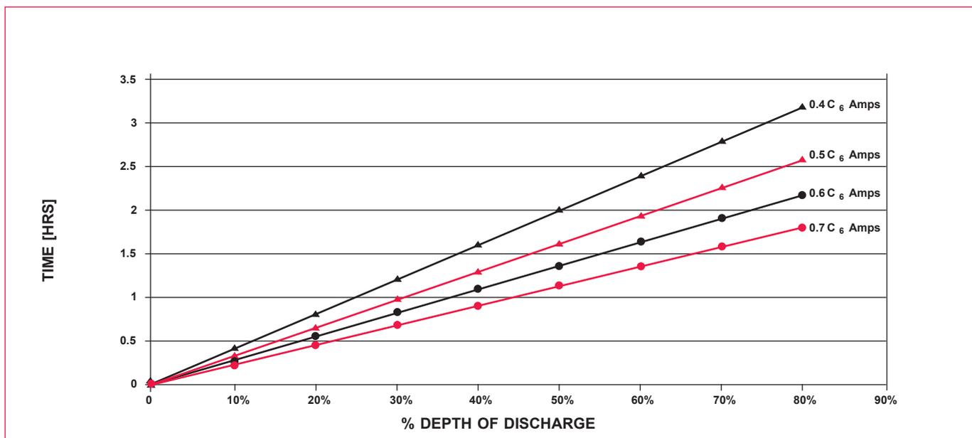
Figure 4 – Recharge time – return 100% of discharged Ah's
