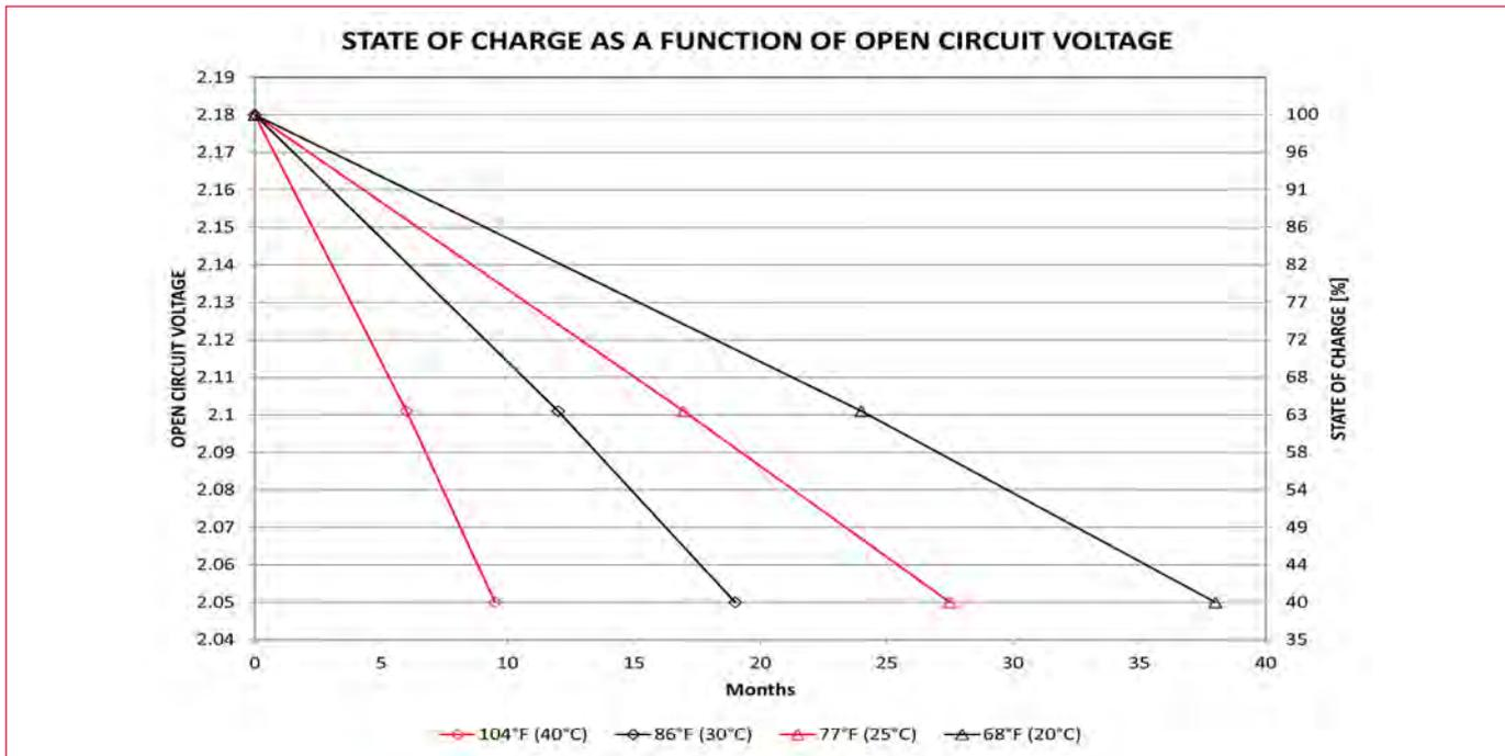
Figure 2 – Open circuit voltages state of charge
