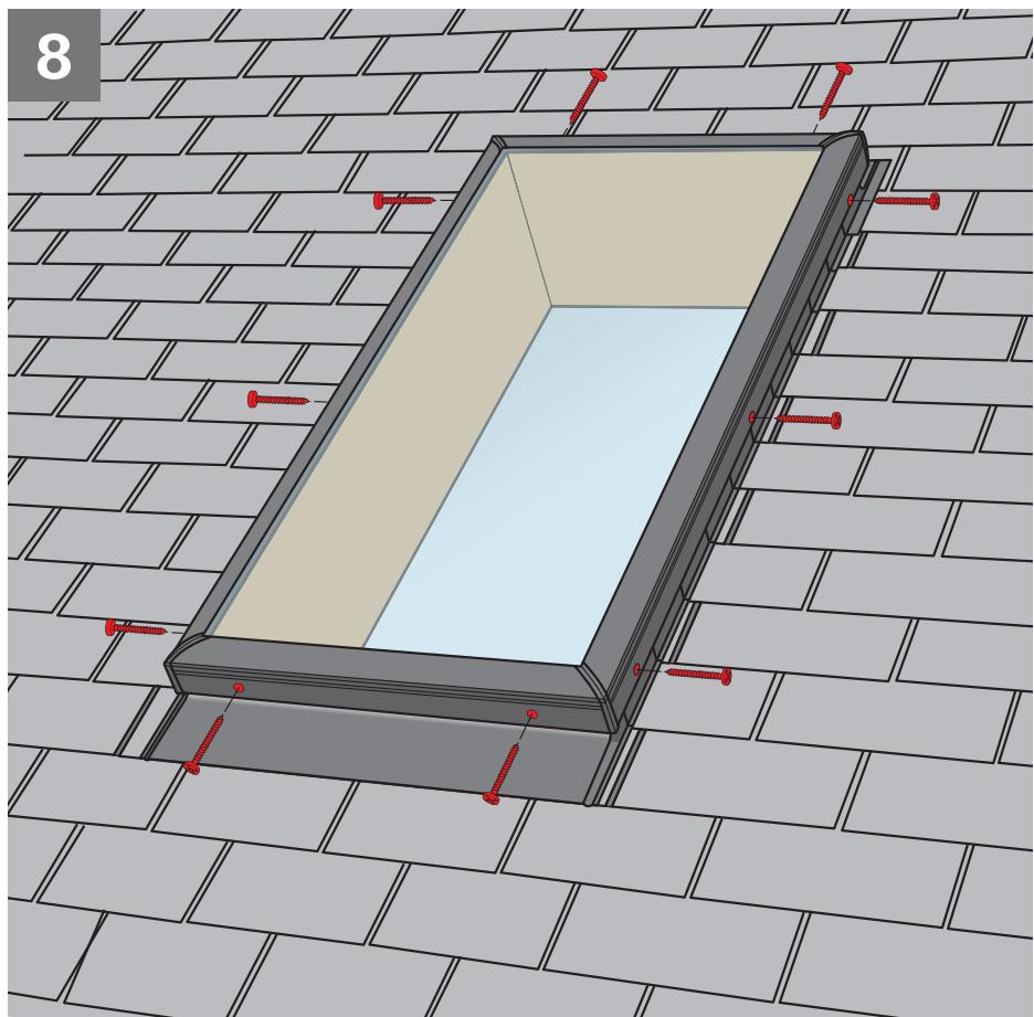
**ENGLISH:** Center the skylight on top of the curb and secure with #8 1 $\frac{1}{4}$ " (4.2 x 45 mm) pan head stainless steel screws provided. Screws will penetrate the curb by at least  $\frac{3}{4}$ " (19 mm).
