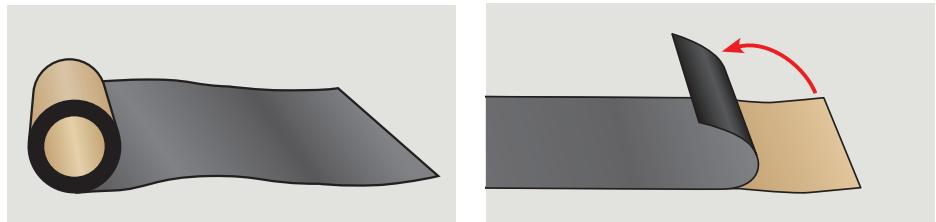
**ENGLISH:** To ensure waterproofing, skylight curbs shall be completely wrapped in VELUX adhesive skylight underlayment as indicated. Underlayment must be applied before installing the flashing.
