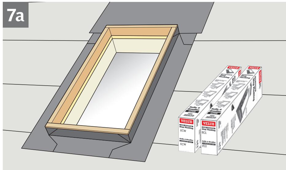
**ENGLISH:** For thin roofing materials, use flashing ECL. ECL is designed for roof pitches 10°-60° (2:12 - 21:12).
