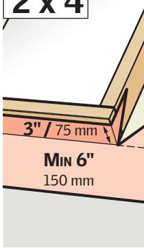
**ENGLISH:** Wrap the bottom and the corners of the skylight curb with the underlayment and create water-shedding laps over roofing underlayment.
