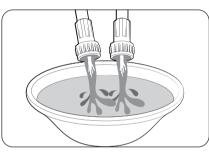
3. Put the other ends of the hoses into a bucket, and then open the water taps for 10 - 15 seconds to remove impurities. When done, close the taps.
