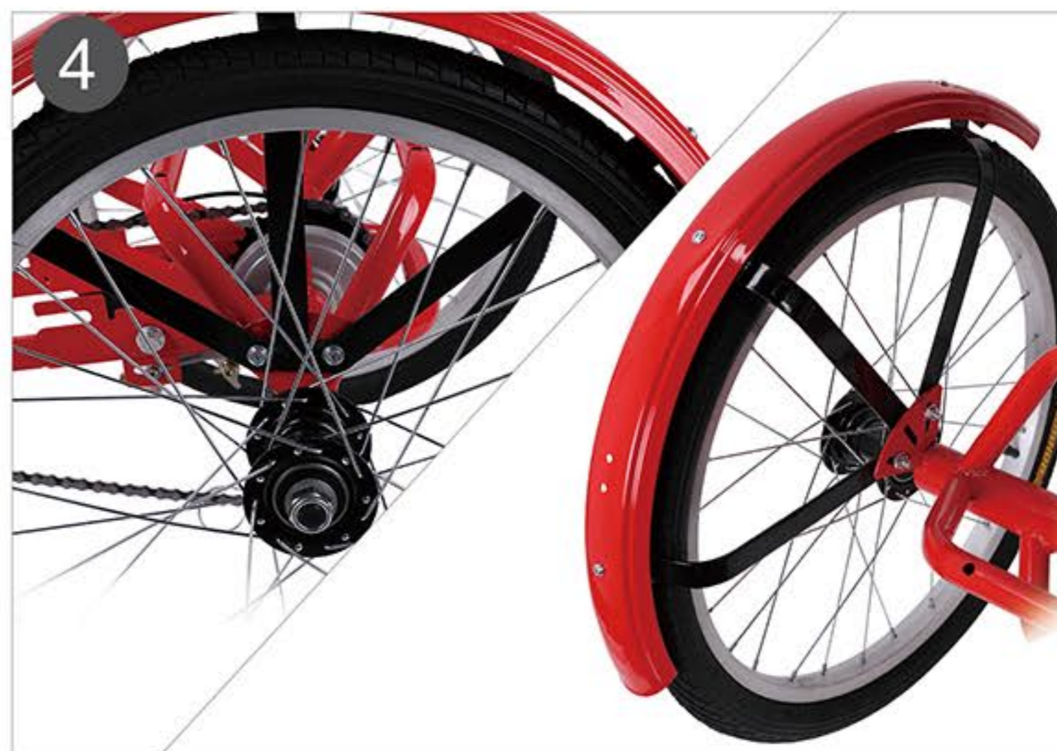
4. Finished, the effect shows. Note: If the fender is not in the correct position, adjust the screw position.
