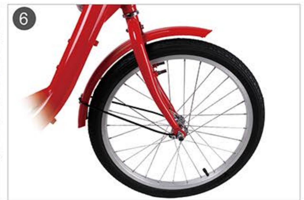
6. Make sure there is no friction between the tire and the fender
