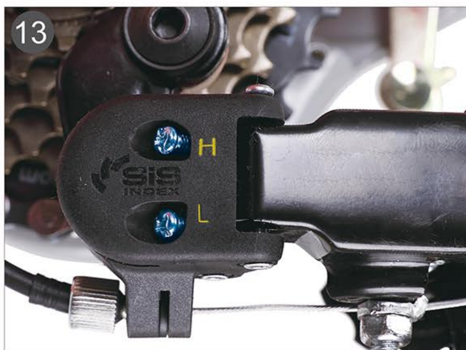
13. If there is a shifting fault, adjust by screws (H and L).
