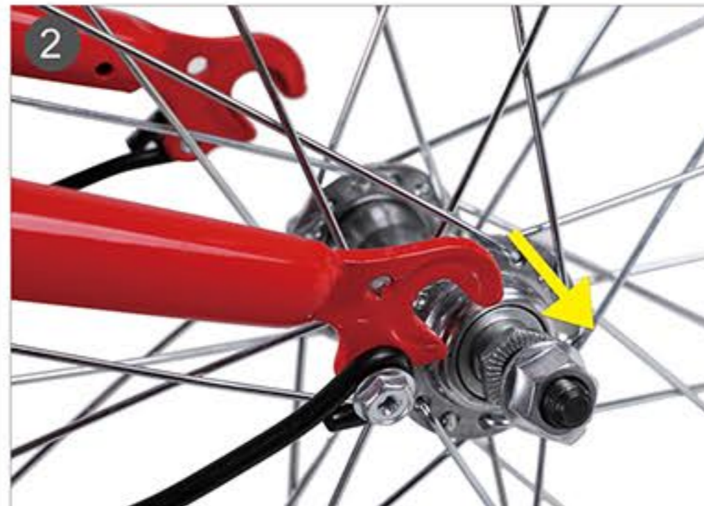
2. Let the screw hole on the front fork catches the bolt.
