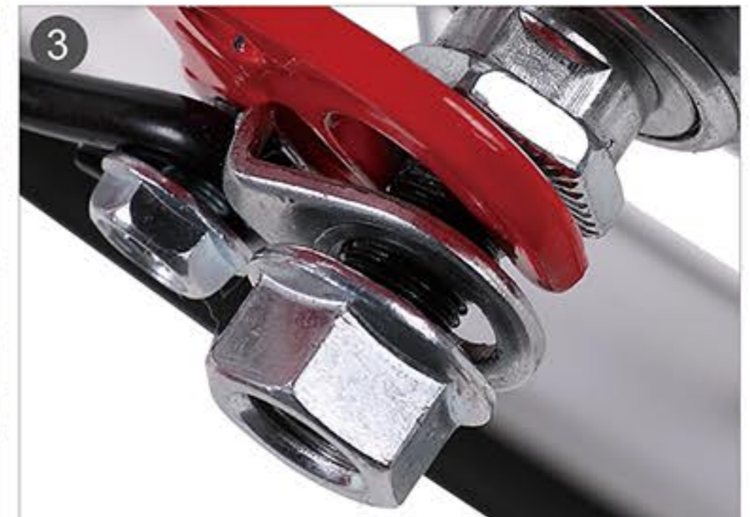
3. The fork is inside, the washer is in the middle, the nut is outside.
