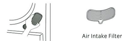
Slightly push upwards with your thumb until the latch hook disconnects, then remove.
