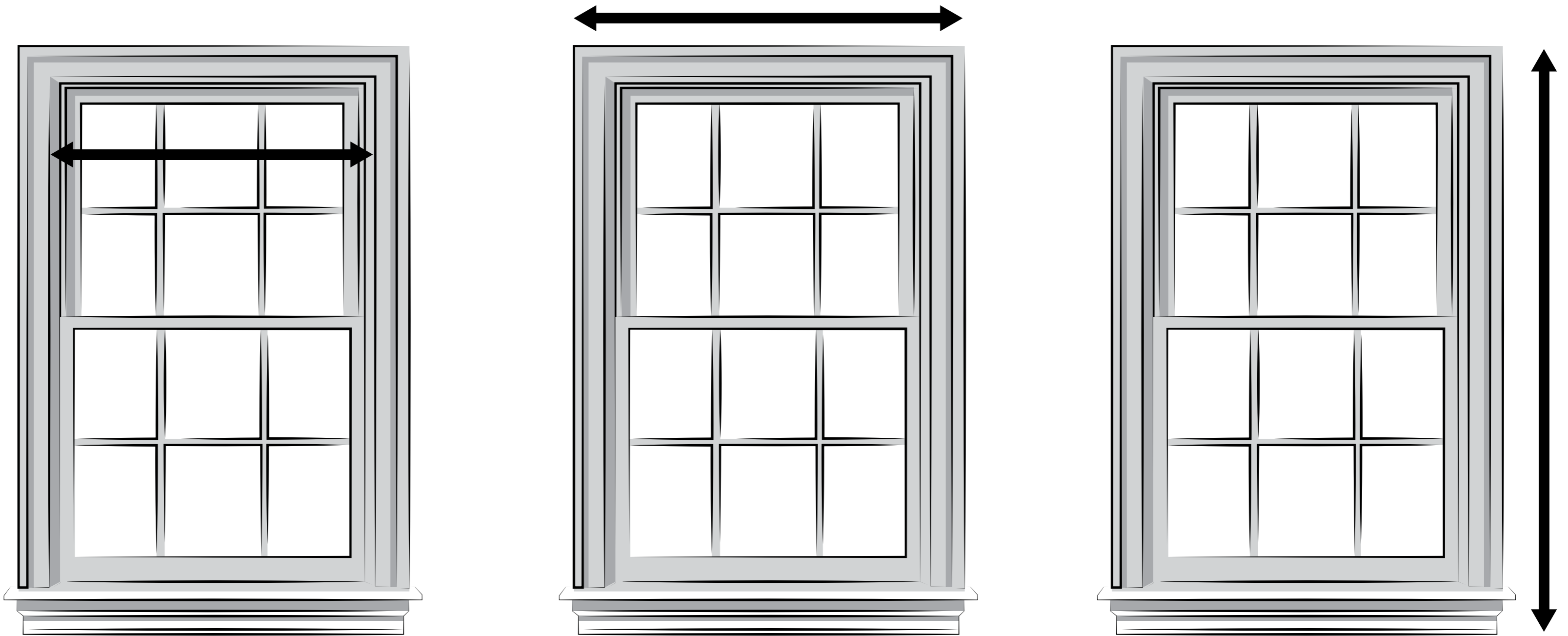
Measure here for the width inside the frame
