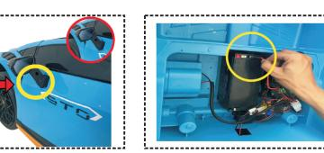
Install "2": Line up "2" with the holes on both sides of the car and press down.
