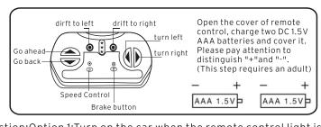
Connection:Option 1:Turn on the car when the remote control light is on. If the light is flashing, everything is okay.
