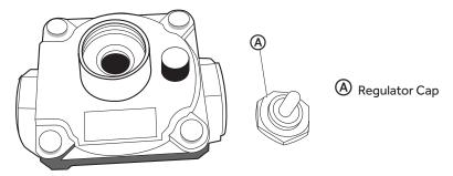
2. Remove the retainer pin that is currently positioned for use with Natural Gas.
