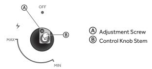
1. Light one burner and turn the control knob to the lowest setting.
