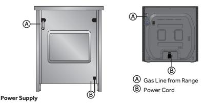
**IMPORTANT:** An electrical outlet in the floor, may be either recessed or surface mounted, but an electrical outlet in the wall must be recessed to make the connection.
