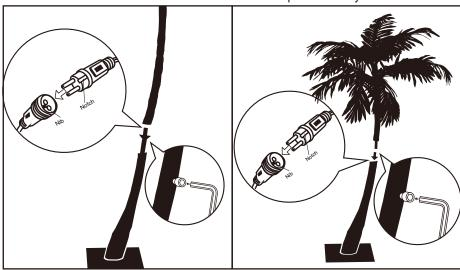
4. Connect with the Solar Panel. Fix the base by ground stakes.
