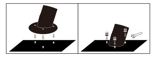
3. Find the wire joints inside the upper & bottom trunks. Connect the joints, insert the upper trunk into the bottom one and fix the trunk with the screw preinstalled by Allen wrench.
