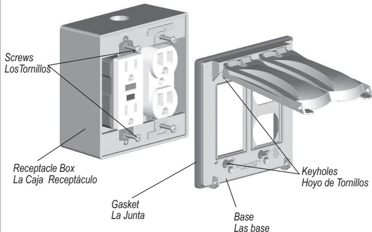
**Turn off power to receptacle.** Configure base as shown on other side. Back-out box screws. (Note: Make sure that box is flush or slightly behind the finished surface and that receptacle is flush with the finished surface in accordance with NEC 406.4 and 314.20.) Place gasket over the screws. Using keyholes, place base over screws and against gasket. Tighten screws. Do not over-tighten mounting hardware.
