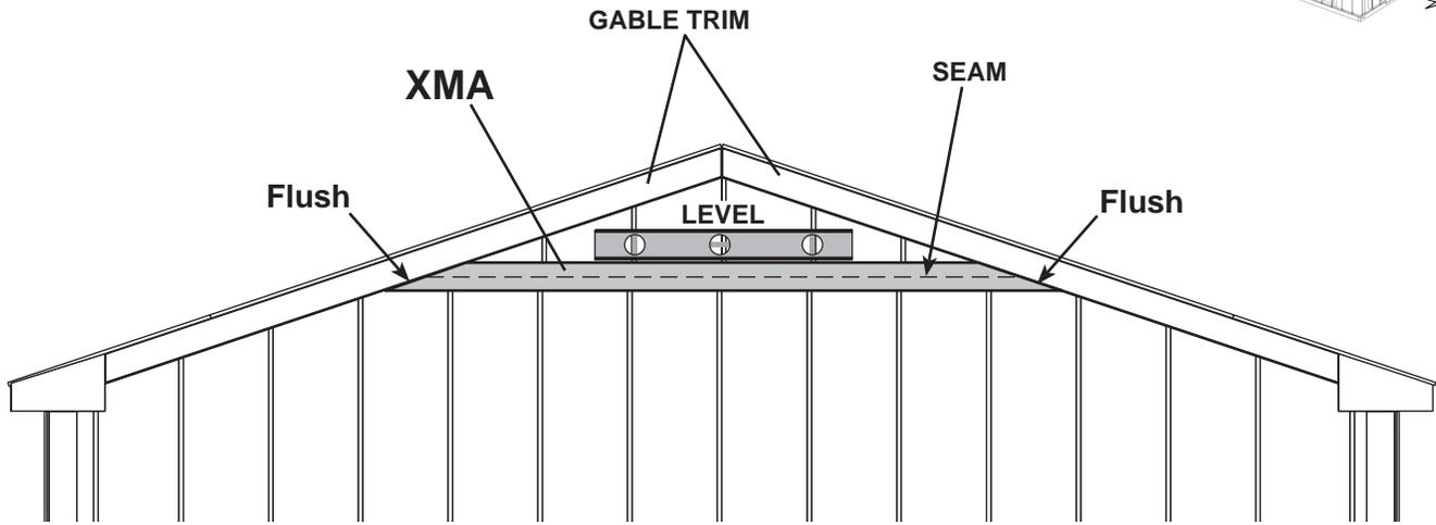
**2** From the *inside*, fasten **XMA** with 3/4" screws, in the pattern shown.
