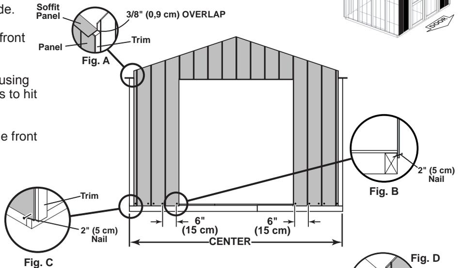
**2** Be sure the measurement between the panel edge and the trim is the same along the entire length. Then secure with (1) 2" nail in the upper corner (**Fig. D**).
