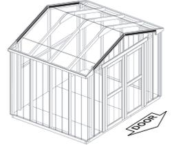
**2** Install 2nd **CDD** flush to panel edge and flush to installed **CDD** (**Fig. A**). Secure trim with (8) 1-1/4" screws from inside. Install (2) screws at seam (**Fig. B**).
