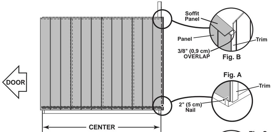
**2** Ensure the measurement between the panel edge and the trim is the same along the entire length.
