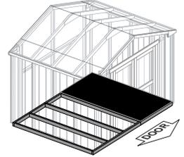
**2** Move to the opposite end. Using the long edge of the panel as a lever move the panel side-to-side until the top corner is flush to the floor frame (**Fig. B**). Secure panel with 2" nails in the corners.
