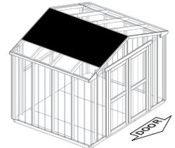
You must square the roof by attaching (1) panel fist. You will use the panels' long edge as a lever to bring your roof into square. Commonly known as "racking".
