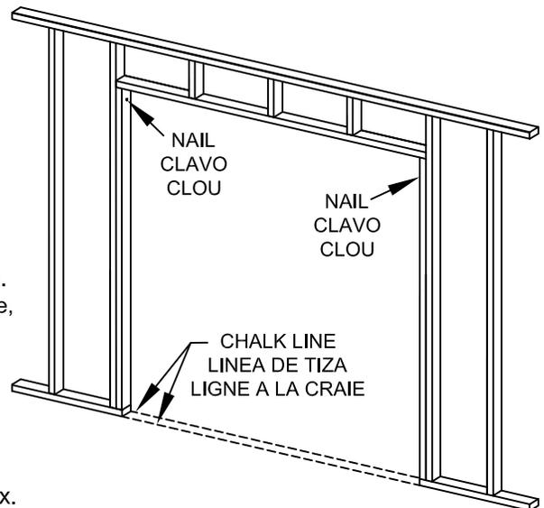
**4** Slip slots in Frame Header End Plates over nails in rough studs. LEVEL HEADER. Set nails and drive nails through remaining holes in end plates. (If you have the 2/6" (761mm) or Universal Frame and using another size door, see cutting instructions on page 4.)
