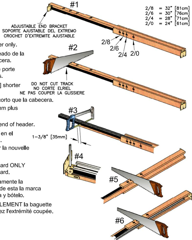
Cutting header for other than standard door width: Measure door width and multiply by 2. Add 1" (25mm). Mark header and cut (Step #2). Cut track (Step #3). Measure door width. Add 1" (25mm). Mark header Trim board and cut (Step #5 & #6).
