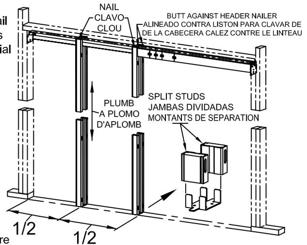
**6** Apply desired wall material. Wall material is brought clear to edge of opening. WARNING: Use nails no longer than necessary. Nails must not protrude into pocket or door will be damaged. To provide a firm nailing surface, slip a 2-1/8" (54mm) wide board between Split Studs temporarily.
