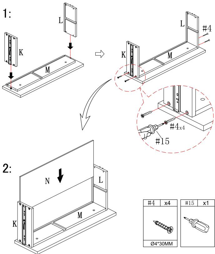
1.Connect the (J) and (L&K) using screw #4 , and tighten it with screwdriver #15.
