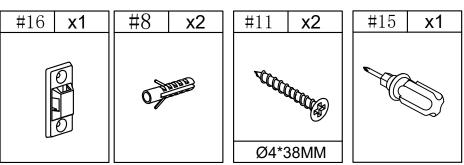
1. Mark the position on the wall, that corresponds to the location of bracket #16 on the panel (H). Drill and insert the expandable screw #8 by hammer.
