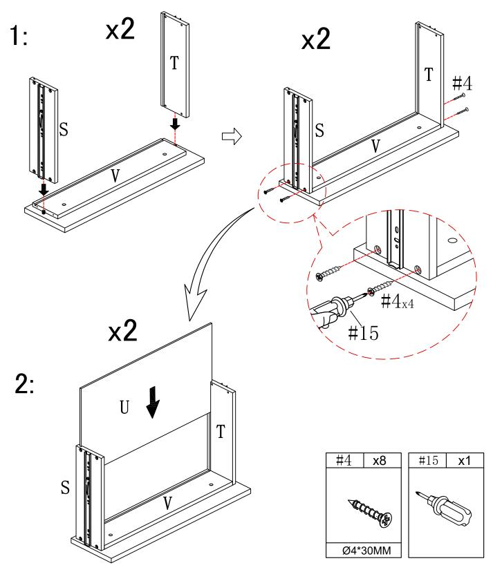
1.Connect the parts(R) and (S&T) using screw #4 , and tighten it with screwdriver #15.
