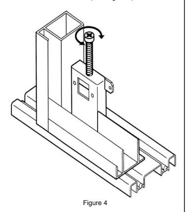
B. Slide the back Mirrored Panel (#1) to the opposite wall. Adjust the alignment of this panel by turning the adjustment screw on the Steel Wheel Assembly (#14) nearest the wall until the door aligns straight, up and down, with the wall.
