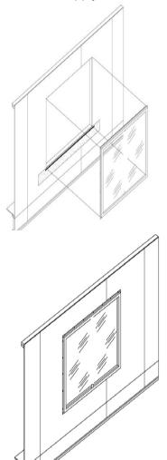
Use caution to avoid covering any window weep holes with sealant, paint or any other obstructive material
