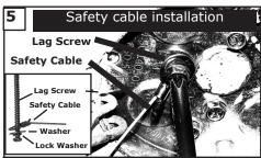
For Canadian installation and for USA fan and light kit combinations over 35 lbs, in both flush and downrod mode the safety cable must be installed into the house structure beams using the 3" lag screws provided. Make sure that when the safety cable is fully extended the leadwires are longer than the cable and no stress is placed on the leadwires. **Note**:If Installing The Secondary Support Safety Cable in the U.S., Do Not Remove Knockouts In The Outlet Box.
