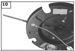
Loosen the two screws and washers across from each other on the ridge of the mounting plate. Remove the other two screws and lock washers. Save for later use.
