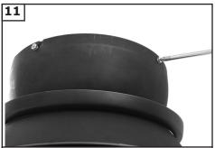
Lift the motor housing up aligning the L shape holes with the screws and washers on the mounting plate. Turn the housing clockwise to hold in position. Install the other two screws and washers previously removed securely.
