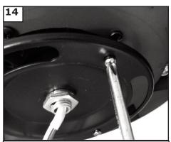
Loosen 2 screws and remove 1 screw from motor plate. Save removed screw for use later.
