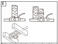
Before installing this fan make sure the outlet box is properly installed to the house structure. To reduce the risk of fire, electric shock, or personal injury, mount to outlet box or supporting system acceptable for fan support. (Mounting must support at least 35 lbs.)
