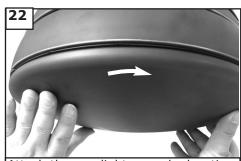
Attach the non light cover by locating dimples in the light fixture with the grooves in the non light kit cover and twist clockwise till tight. **WARNING:** Make sure light bulb is not installed when using this cover.
