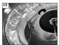
Install by twisting clockwise, add 1 screw removed step 14 to switch housing plate. Tighten the 3 screws securely.
