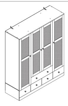
Install anti-tipping device as shown.
