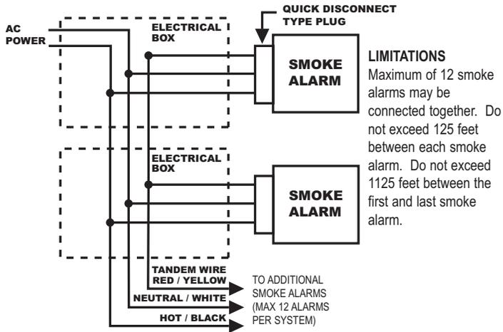
1. Run a minimum of 16 gauge, 3-conductor cable, plus ground (4 wires) to the first junction box from a power supply and between all smoke alarms that are to be connected together. Use ANSI/UL listed Class 1 wire. Power limited cable for multiple tandem connections are available at many commercial electrical retail stores.
