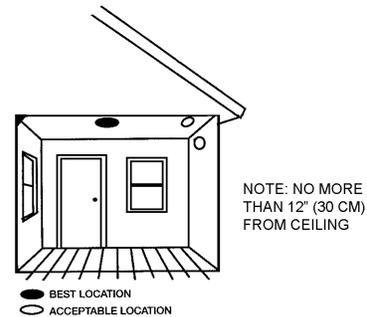
FIGURE 5: RECOMMENDED SMOKE ALARM MOUNTING LOCATIONS.
