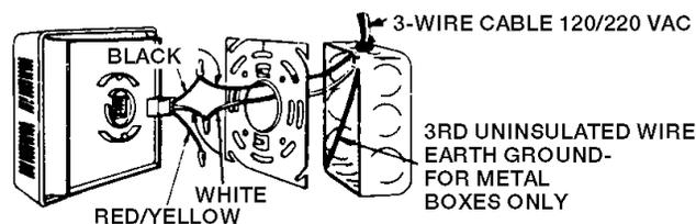
**NOTICE:** RED-YELLOW WIRE: THE RED-YELLOW WIRE FROM THE SMOKE ALARM IS FOR TANDEM CONNECTION ONLY. DO NOT USE, AND DO NOT REMOVE INSULATION CAP UNLESS CONNECTING ANOTHER SMOKE ALARM.
