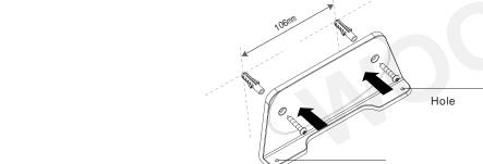
(3)Install battery and place remote control to the hanger.
