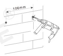
(2)Insert expansion tube into the hole on the wall, install the hanger to the wall with a screw, and paste the double faced adhesive tape on hanger to the wall, tighten the screw.
