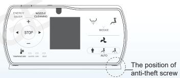
**Notice**: Please do not install and use the product in moist place, such as steam room, and prohibit to place in the space where is easily got wet. In public place, please use screw to fix the remote control with bracket in avoid remote control missing.
