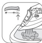
Fill the water tank with untreated tap water up to the max mark and heat the iron to the temperature. Unplug the iron and hold it over a sink horizontally. Hold the steam control into the Self Clean position : steam will now begin to build up. After a few seconds water will emerge from the soleplate, rinsing dirt and scale particles out of the steam chamber.
