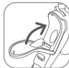
**IMPORTANT** Before filling the water tank, unplug the iron and set the steam control to dry position
