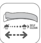
Unplug the iron, pour away remaining water and set steam control to . Open and close the steam control several times to prevent the valve hole into the steam chamber from scaling or blocking up.
