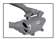
1.Turn the rear cover counter-clockwisely to remove the cover.
