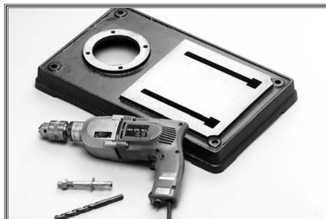
Figure 6. Secure base to floor.
