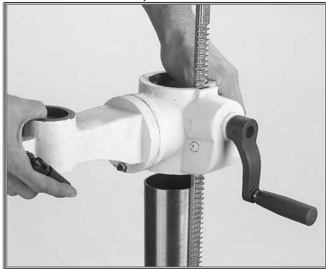
Figure 11. Installing rack and table bracket.
