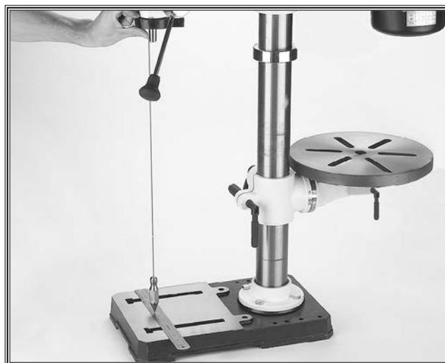
Figure 16. Aligning the headstock.
