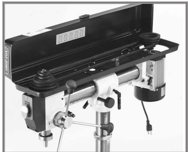
Figure 36. Adjusting belt to desired speed.
