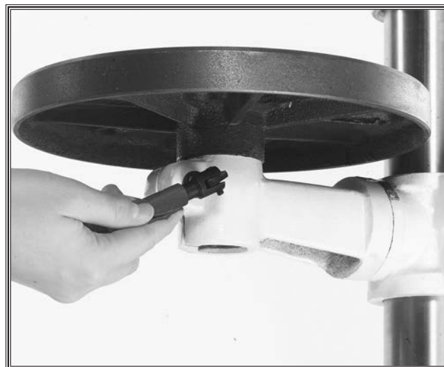
Figure 27. W1669 Table support assembly.
