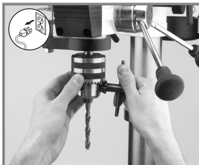
Figure 34. Using the chuck key.
