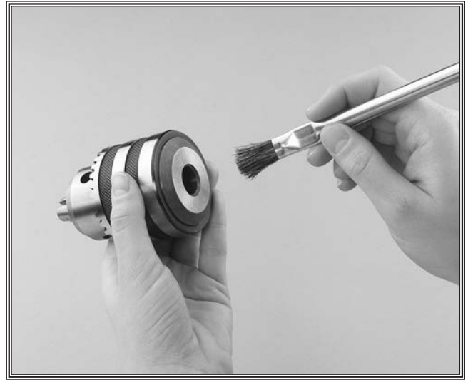
Figure 17. Clean the chuck before installation.
