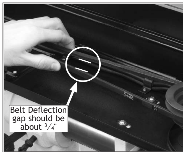
Figure 21. Measuring belt deflection.
