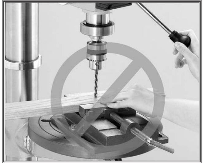
Figure 2. Keep fingers away from spinning drill bits, cutters, and sanding surfaces.
