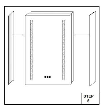
The side panels and cabinets are individually packaged, you need follow the STEP 5 to STEP 7 to install the side panels for hanging walls version, for embedded installation no need install the side boards.
