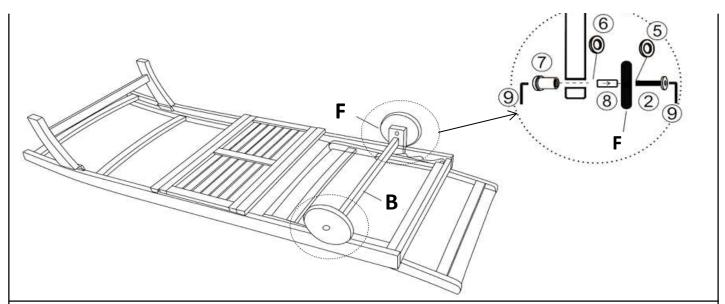
Attach one of Wheel (F) to Back Leg Panel (B) by using Bolt (2), Washer (5), Iron tube for Wheel (8), Washer (6) and Sleeve Nut (7) with Allen Key (9) in sequence as shown on the picture above.
