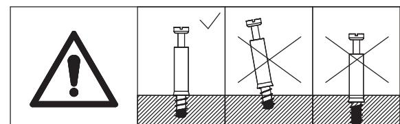
Insert quickfit screw(A) into No.10 and No.20 plate with a screwdriver as shown.
