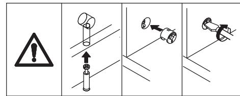
Attach No.3, No.4, No.5, No.6 and No.17 plate with No.2, then turn cam lock(C) in No.3, 4, 5, 6, 17 plates clockwise to tighten as shown.
