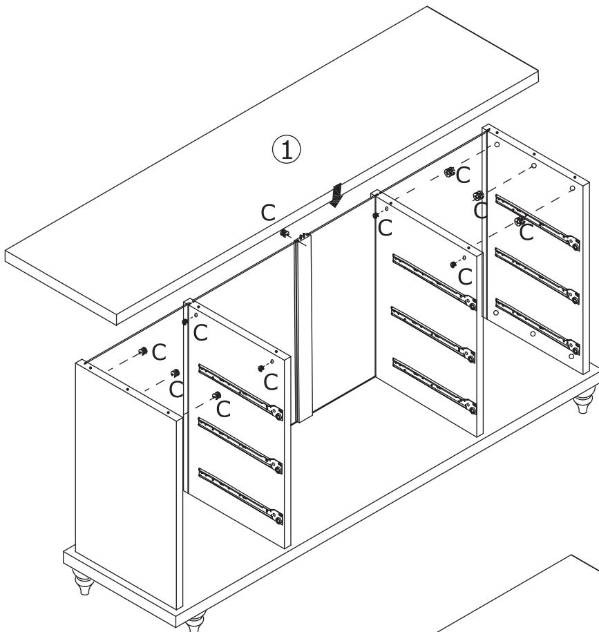
Cover No.1 plate to the top the unit, then turn cam lock(C) in No.3,4,5, 6 plates clockwise to tighten as shown.
