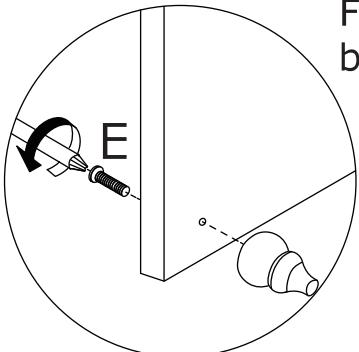
Fix No.18 leg and No.19 leg support to bottom of No.2 plate with screw(E) as shown.
