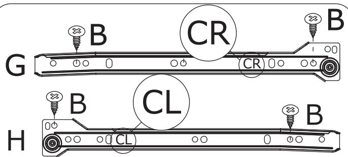
Please note the holes on both sides of the plate are not consistent, just for preventing the plate from being pierced by screws.
