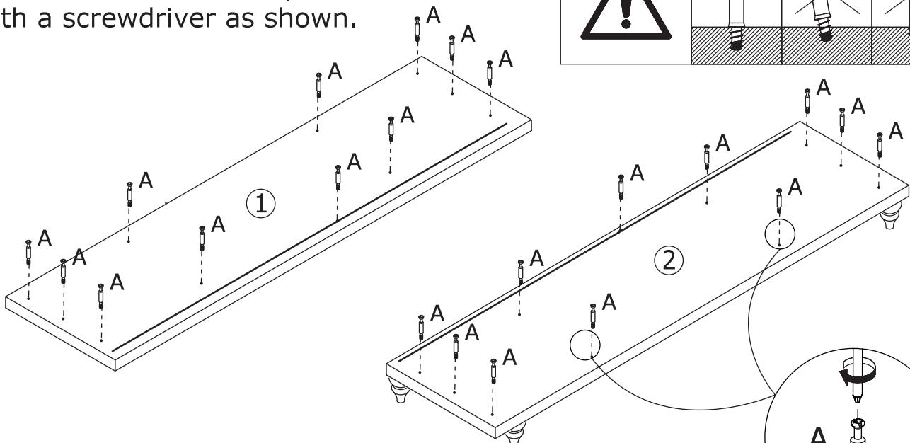
Do not use an electric drill , do not use force during the rotation of the accessories, otherwise it may cause the board to crack
