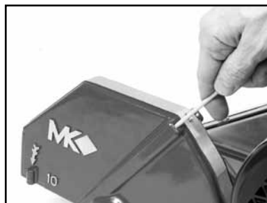
(H) Rod Cooling Channels and recheck flow
