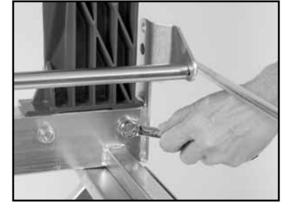
(F) Secure the Post Support by tightening Retaining Bolts.
