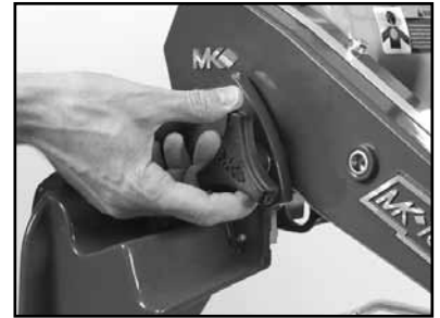
(C) Install the Cutting Head onto the Post Pivot Shaft and install the Adjusting Knob
