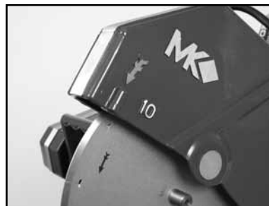
(E) Verify the Blade is seated on the Blade Shaft and direction of rotation is correct
