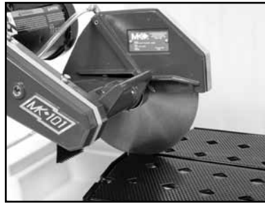
(B) Set cutting depth approximately 1/4 to 1/2 inch below the surface of the Movable Cutting Table
