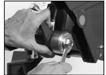
(C) Depress and hold the Shaft Lock pushbutton and remove Retaining Nut and Outer Flange using the Blade Wrench
