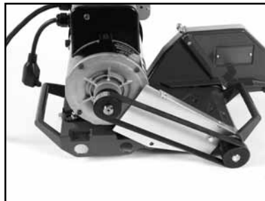
(E) Inspect the Micro-V Belt for cracks, fraying, separation and wear. Go to step H if replacement is required
