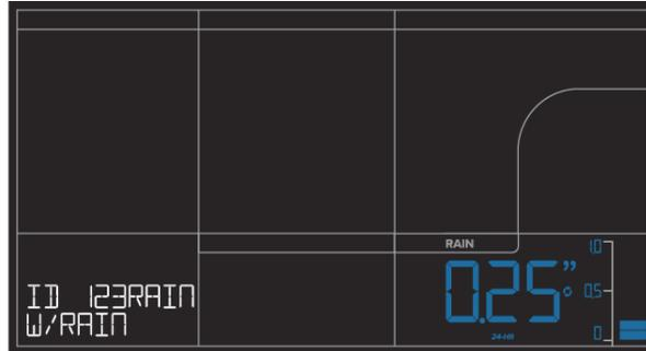
3. While viewing the ID for the sensor you wish to delete, hold down the MINUS (-) button until dashes appear. This will remove the sensor from the display and have it immediately begin searching for a new compatible sensor connection.
