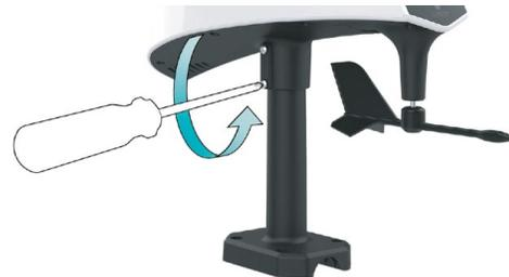
3. Secure the Cyclone Sensor to the Mast by tightening the screws on the side. Double check the Bubble Level to be sure the sensor remains level.
