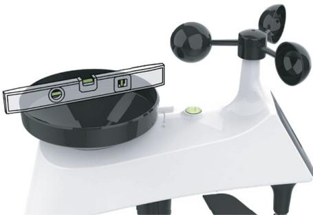
4. Check the Bubble Level to ensure the sensor is level.
