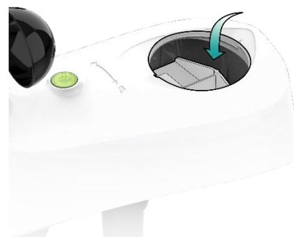
1. Clear any leaves, insects, or other debris to allow the Rain Tipper to rock freely. Check that the drain vents on the bottom are clear.
