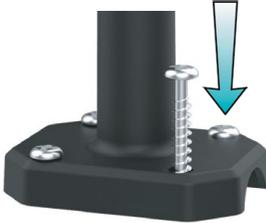
1. Mount the Mast to a flat surface with the four provided screws.
