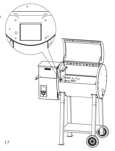
Re-install the temperature probe cover removed in Step 7.
