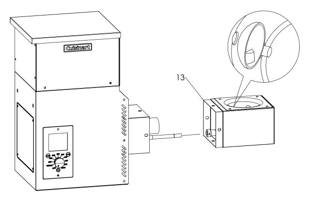
With the hot rod in place, re-install the screw removed in Step 11 to secure the hot rod.
