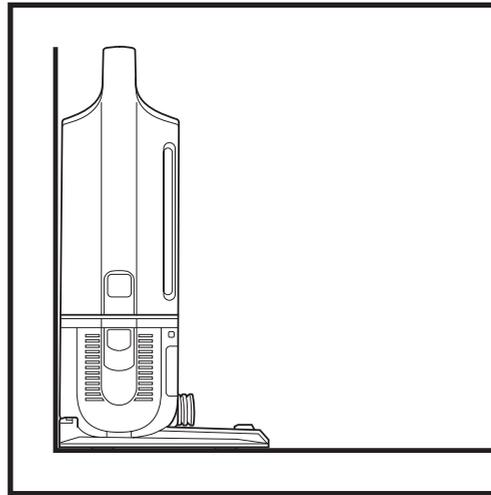
The **Self-Empty Base** charges your robot and holds dirt and debris from up to 30 days of cleaning. Select a permanent location for the base, because every time you relocate it, your robot will have to completely re-map your house.
