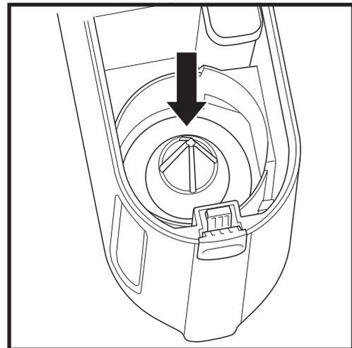
After emptying the dust bin, ensure there is no debris or dust stuck on the filter mesh.
