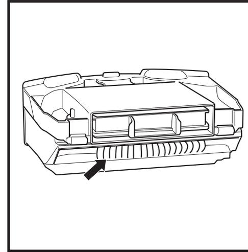
Remove and empty the robot dust bin. Clean any hair or debris off the **Anti-Tangle Comb** on the back of the dust bin.
