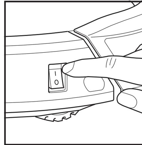
To charge, the **Power** button on the side of the robot must be in the ON position (I). The robot will beep when charging begins.
