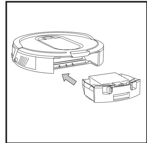
Reinsert the filter into the robot dust bin, then slide the dust bin back into the robot.
