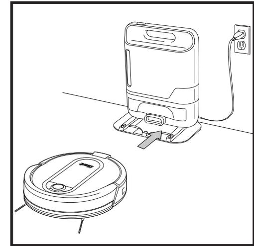
When the cleaning cycle is complete, or if the battery is running low, the robot will search for the base. If your robot doesn't return to the base, its charge may have run out.
