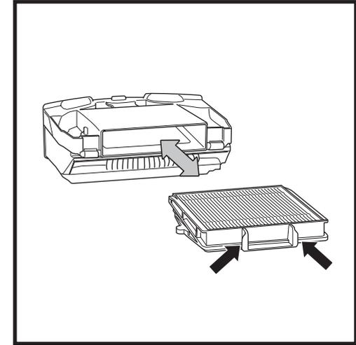
Pull filter out of the dust bin by the tabs.
