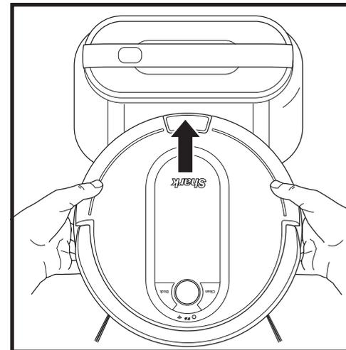
If the robot has no charge and cannot return to the base, manually place it on the base. The base indicator light will flash blue and the robot will beep when charging begins.
