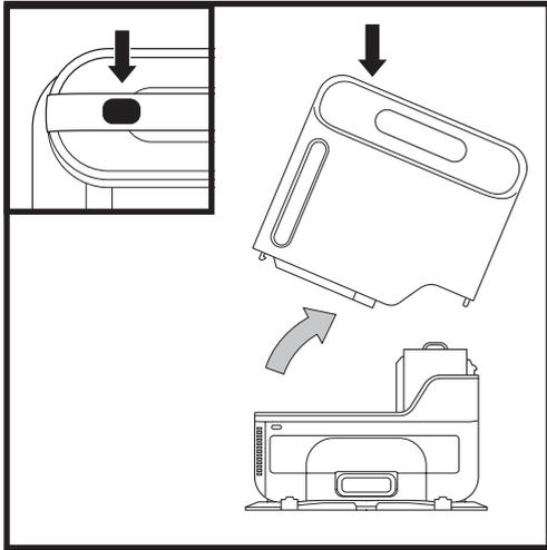
The **Base Dust Bin** holds up to 30 days' worth of dust and debris. Empty the bin when the debris level approaches the max fill line.
