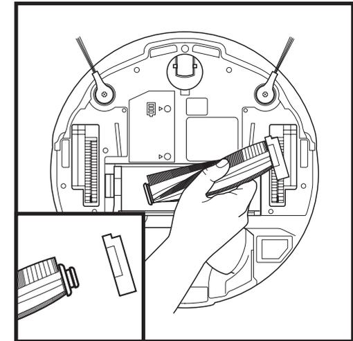
Lift out the brushroll. Remove the cap on the end of the brushroll. Clean off any debris, then reattach cap. Reinstall the brushroll, inserting the flat end first. Close the brushroll access door and press down until both sides click into place.
