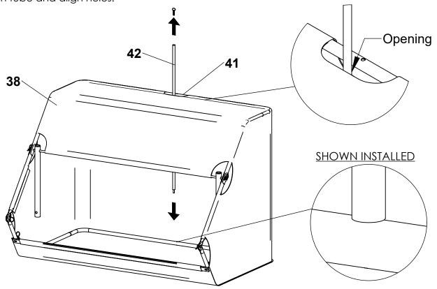
Insert thumb screw that came with Tension Tube Assembly (44) through top Center Frame Tube (41) and screw into top of Tension Tube.
