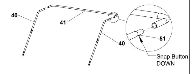
First, Place top frame assembly into Hopper Bag (38). Second, Install Clevis Pins (45) through Top Frame Tubes (40) and Bottom Frame Tubes (39) and secure with Hairpins (49). 9 40 38 49 45 39 49 Frame into Hopper 45 Snap Button Down
