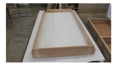
If a brad nailer is available, apply the wood glue sparingly to the first corner and use the brad nails to hold the threshold in position while you pre-drill and countersink the holes for the screws.
