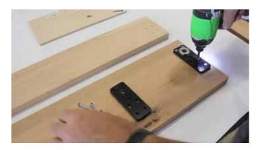
Attach the upper flush mount hinge to the top threshold using 4 - 1" screws. Chamfered sides should be facing up.
