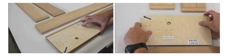
Drill the designated holes for an in-swing or out-swing configuration, but do not drill the large hole on templates out-swing pattern into the bottom threshold. This large hole will only be drilled on the top threshold piece.
