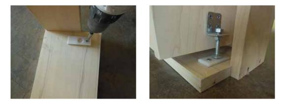
NOTE: Make sure that the Poly Wedge is pointing in the right direction as to have the Catch Bolt slide up the Poly Wedge to its final resting position.
