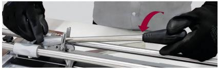
2 - Take the old Scoring Wheel out of the toolholder and replace it for a new one;
