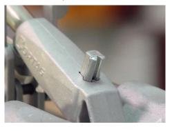
3 - Twist the handle clockwise to tighten the new Scoring Wheel.
