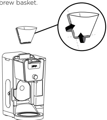
**NOTE:** Fold the paper filter along the seams, open the top fully, and firmly press it into the brew basket, making sure it is fully seated.
