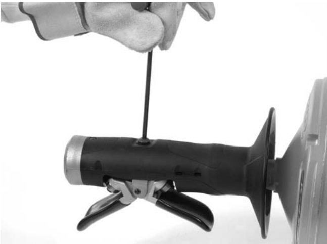
Figure 12A – Removing AUTOFEED Screw
