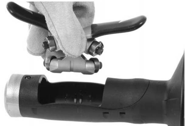
Figure 12B – Removing AUTOFEED Mechanism From Housing
