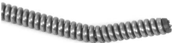
Figure 15 – Bend At Cable End
