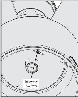
To switch the direction of air flow, move the reverse switch to the opposite position.
