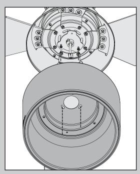
Feed the wire plug through the center hole of the hood, then wrap keyhole slots around the screws and twist counterclockwise.
