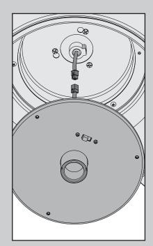
Connect the plugs from the fan and lower switch housing. Make sure to line up the colored markings on the connectors.
