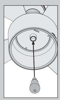
Install the bulb into the socket. When necessary, replace with bulb of the same type and wattage.
