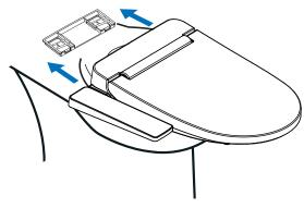
Secure the remote control holder to the wall with screws or peel off the double-sided tape sticker on the back of the remote
