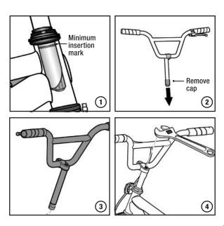
**WARNING:** Do not over tighten the stem bolt. Over tightening the stem bolt can damage the steering system and cause a loss of control.
