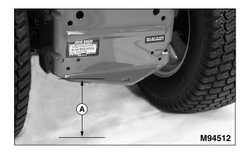
1. Measure length (A) from ground to top of hitch plate with tractor parked on a level surface.
