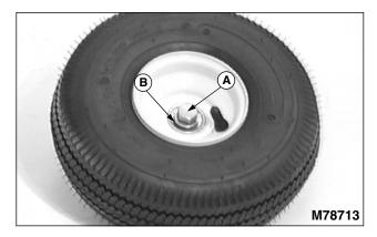
1. Install  $1/2 \times 3-3/4$  in. hex bolt (A) and 1/2 in. flat washer (B) on valve stem side of wheel hub.
