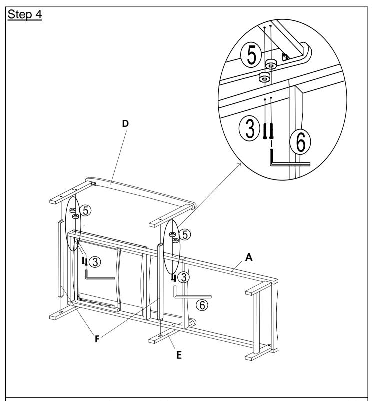
Align the Tenon of Leg Support Bar(F) into the Mortises of Right Armrest Frame(E). Then position Mortises of Left Armrest Frame(D) onto Tenon of Leg Support Bar(F) as shown above.
