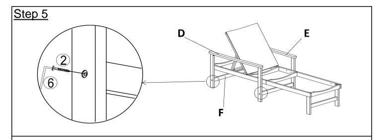
With the help from your adult partner, turn pre-assembled in step 4 right side up Affix the Left Armrest Frame(D) to Leg Support Bar(F) by using Screws( $\bigcirc$ ) with Allen Key( $\bigcirc$ 6) as shown above.
