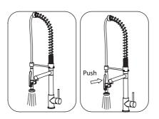
To activate sprayer, turn on water with lever and squeeze sprayer
