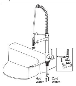
Connect and tighten waterlines (J) to angle stops. Turn on the angle stops and check for leaks (DO NOT TURN FAUCET ON)
