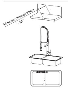
The minimum distance between the faucet hole and the wall should be 3.5"
