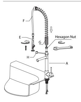
Secure spray hose (F) to faucet body (A). Insert spring (G) into sprayer holder (H). Connect spray head (E) to spray hose (F)
