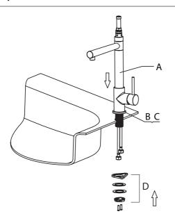
Insert faucet body (A) into hole on deck or sink with base (B) and base o-ring (C) attached. Attach mounting hardware assembly (D)
