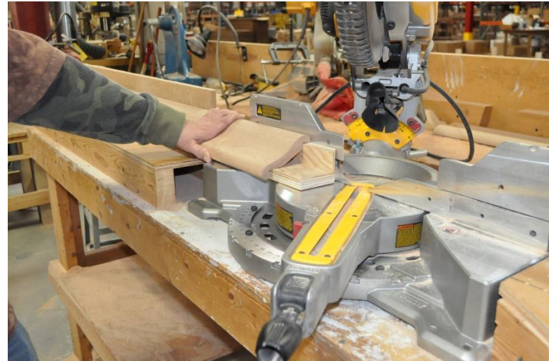
Bar rail in jig at same attitude as installed
